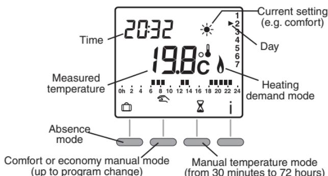
When starting up, the temperature measured by the thermostat is displayed (the symbol appears above the °C).
